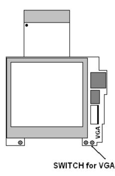
To select between internal LCD or VGA output, connect a switch at the **lower right pad** of the GBC mod kit: **VCC 3.3V** (logic '1') is internal LCD and **GND** (logic '0') is VGA.
