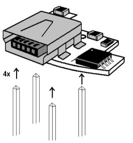
After soldering the pins to the USB charger PCB, you can put the USB charger PCB into the existing holes of the GBC power jack and solder them.
