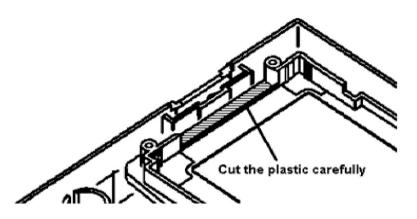
You need to cut a little bit of the case near the power switch (see picture).
